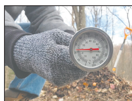
At 48°F, this small compost pile doesn't provide enough insulation for its core to reach high temperatures. -Photo by Francine Wizner
